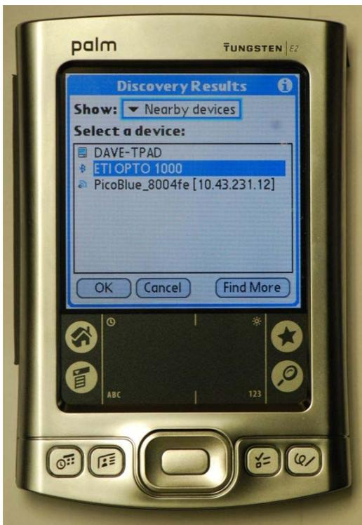
11. Commander is now ready to be used. Go to the Parameters screen and press Read. The Palm will connect to the Bluetooth module (the blue light should become solid while it is communicating with the Palm). Refer to the Commander documentation for additional information about the software.
