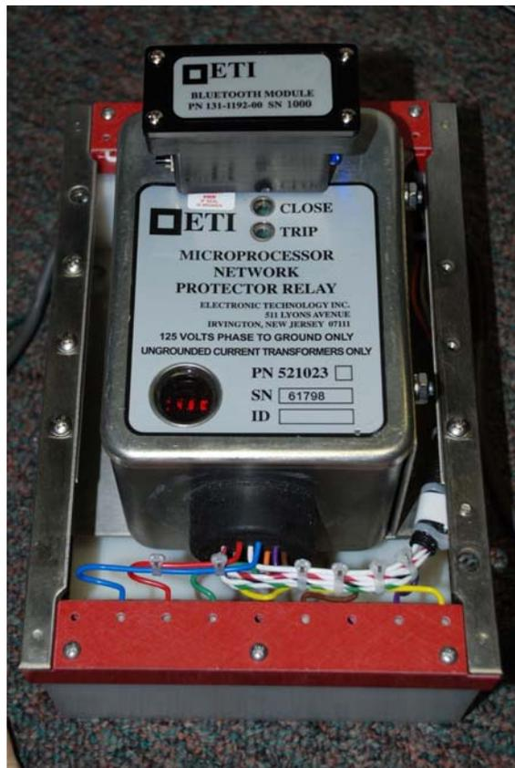
3. Take note of the serial number of the module (in this example it is 1000). This number will be used later to identify the module on the Palm.
