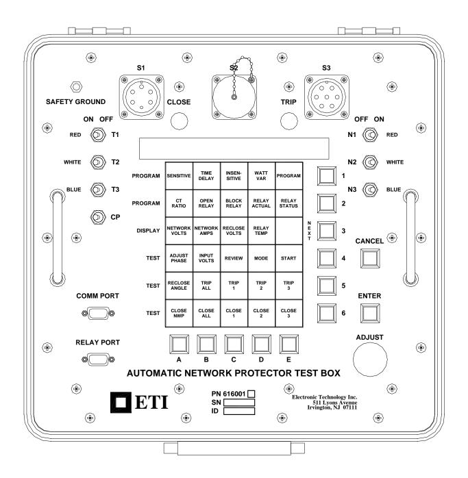
**Figure 1: ETI Automatic Protector Test Box Faceplate**
