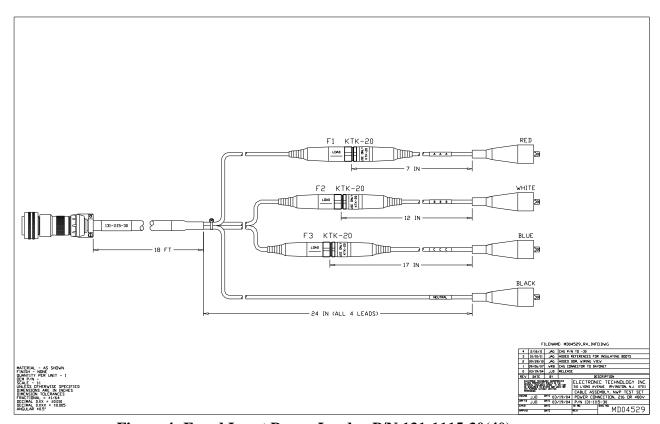
Figure 4: Fused Input Power Leads - P/N 131-1115-30(40)
