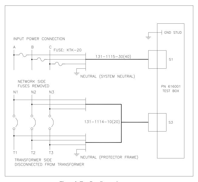
**Figure 2: Test Box Connections**
